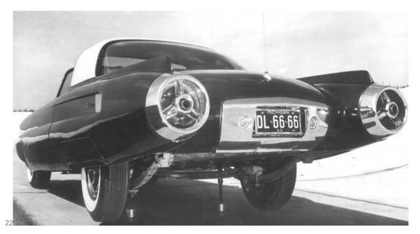
All the gizmos and the revamped steel body not only added a severe load to the electrical system but also plenty of weight overall. Pacific upgraded the car to 12 volt with circuit breakers to handle the electrical load and had to have the tires specially made and many extra gussets placed in the frame to handle the car's 6,300 or so pounds.
